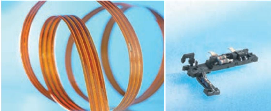
Axon' Cable engineers flat flexible cables for connecting different parts of batteries or inverter systems converting direct current into alternating current. Insulated with polyimide, they resist high temperatures of up to 150°C. The cable's flat configuration saves space in the engine cell. This is an ideal solution for systems requiring energy dissipation.
