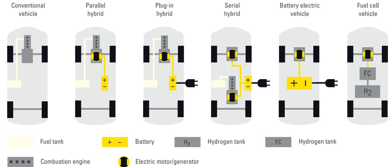
Figure 2: Diversity of e-mobile drive concepts compared to conventional drives (Source: Structure Study BW<sup>®</sup> mobil 2011 – Baden-Wuerttemberg on the way to electric mobility)
